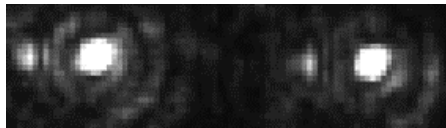
Fig. 1: Camera image of two silica nanoparticles (diameter of 210 nm) trapped at a distance of around 5 \mu\text{m} .
